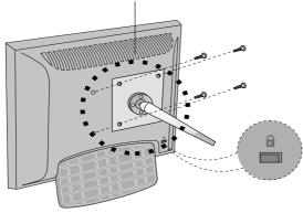
Kensington Security Slot- optional Connected to a locking cable that can be purchased separately at most computer stores
